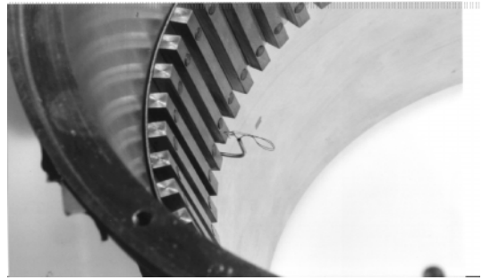
Fig. 2. Picture representing the fixed probe and the inner wall of the cylinder in which the flow takes place, on which the series of square bars is fixed.
